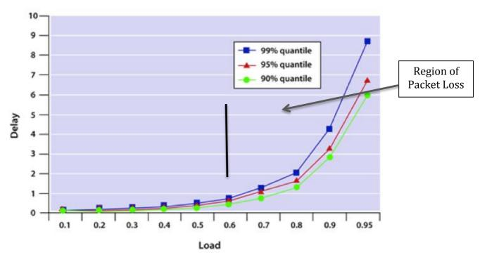
Figure (i) Relationship between Network Delay and Loading
